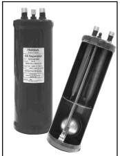
temperature most of the time. If it is hot all the time, this is an indication that the float assembly inside the oil separator may be stuck open and allowing hot discharge vapor to enter the compressor's crankcase. This can lead to excessive crankcase pressures, overheating, and serious damage to the compressor.
