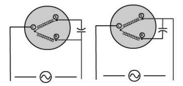
If this solves the problem, it may be only a temporary fix as more than likely the defect within the compressor will cause it to once again lock up.
