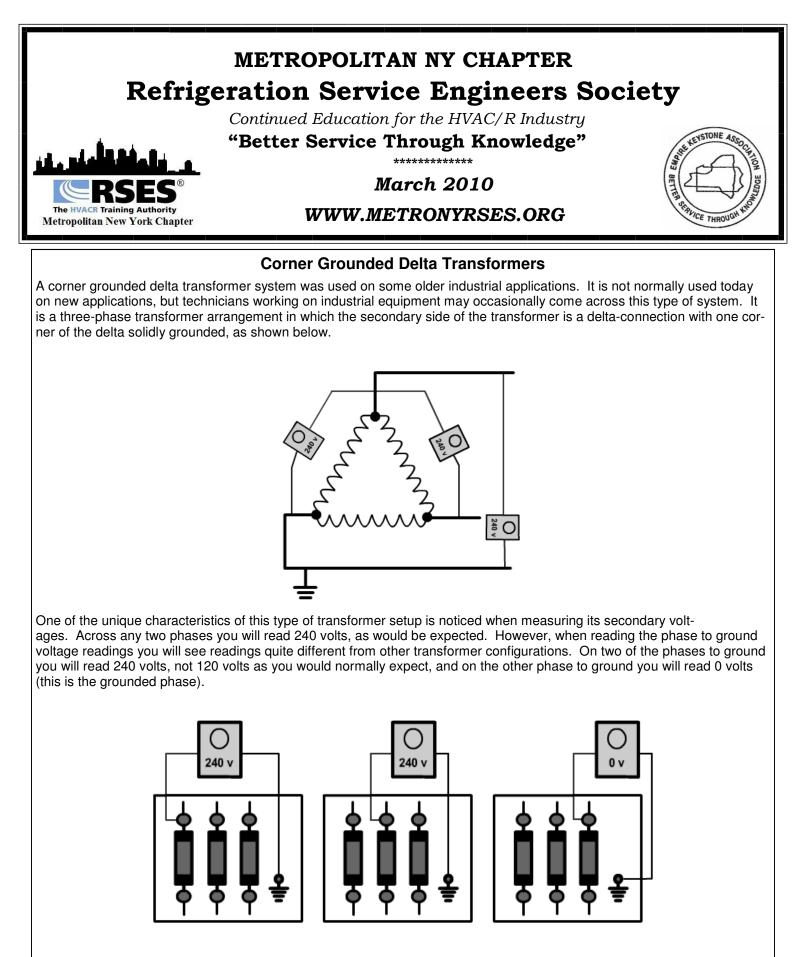
If you encounter this type of system, do not misinterpret these readings as a problem. It is simply the characteristic of its design.
