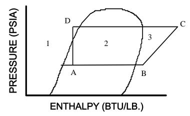
The pressure enthalpy diagram is a useful tool to predict system operation in a typical vapor compression refrigeration cycle. Every refrigerant has its own pressure enthalpy diagram. The lines of the diagram above represent the processes by which the refrigerant goes through a theoretical refrigeration cycle. This diagram assumes no process drop in either the suction or liquid lines.
