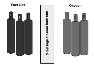
The safe minimum distance between stored fuel gas cylinders and any flammable material is 20 feet or separated by 5 -foot wall with a 1/2 hour burn rating.
