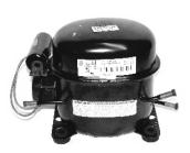
resistance check on the compressor, he will find that the resistance from common to run and common to start to be infinite, and he may interpret this to be an open winding in the compressor. However, if the compressor was allowed to cool down and the internal overload reset, the technician may find the compressor will start normally and will not need to be replaced. The real problem as to why the compressor overheated will need to be identified and resolved.
