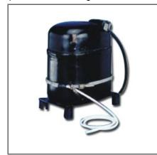
To prevent migration from occurring, it is common practice to keep the oil at a higher temperature than the refrigerant in the rest of the system during the off cycle. This is usually done with some type of resistive crankcase heater.
